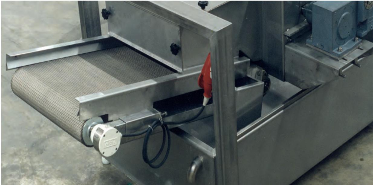
**BS-KK** wide spiral belts normally have to be driven, tensioned and guided by means of plain rollers. In many cases the position of the belt has to be controlled and one or more rollers are executed as dynamic steering rollers. Belt speeds from 0,5 m/min up to 60 m/min are possible.
