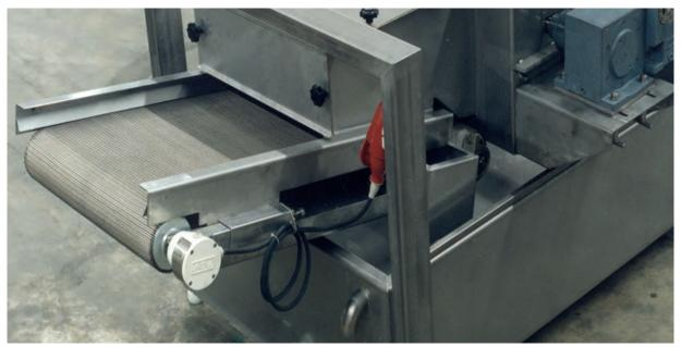
**BS-KK** wide spiral belts normally have to be driven, tensioned and guided by means of plain rollers. In many cases the position of the belt has to be controlled and one or more rollers are executed as dynamic steering rollers. Belt speeds from 0,5 m/min up to 60 m/min are possible.
