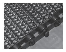
These belts are often used in freezing, cooling, frying or cooking machinery. Or in conveyors where the belt is wide and the length is short. Because this belt has a chain, strong cross rods, side plates and flights are easy to mount on. There are many possibilities in the execution of the chains and the meshes.
