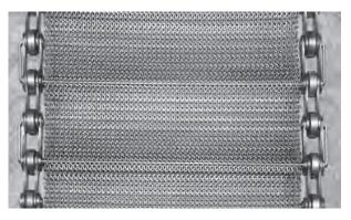
This tight spiral belt is equipped with a 2" hollow pin roller chain. It is often used in (bottle)washing machines, filtrating the water and carrying paper or broken glass out of the installation.
